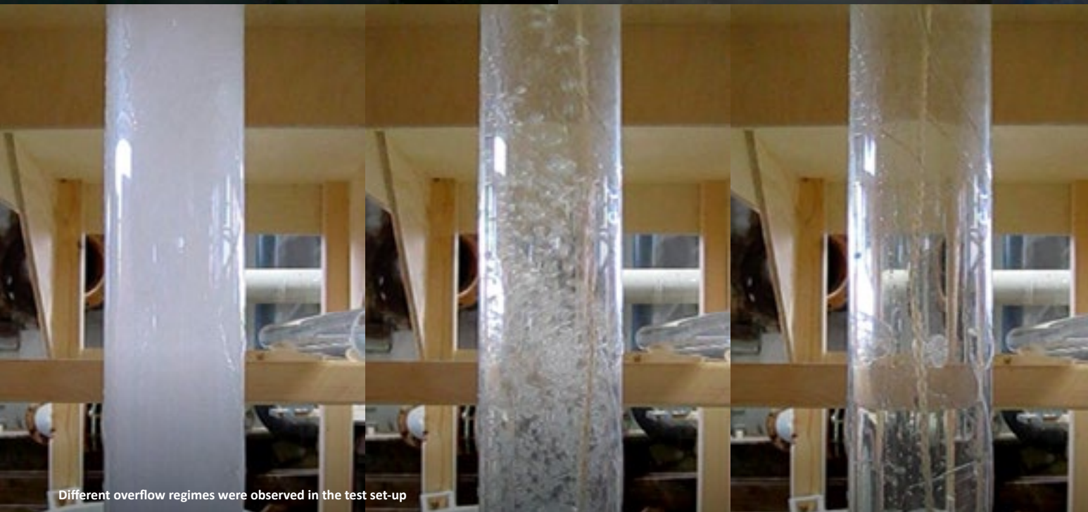
Air enclosed in the overflow during dredging
