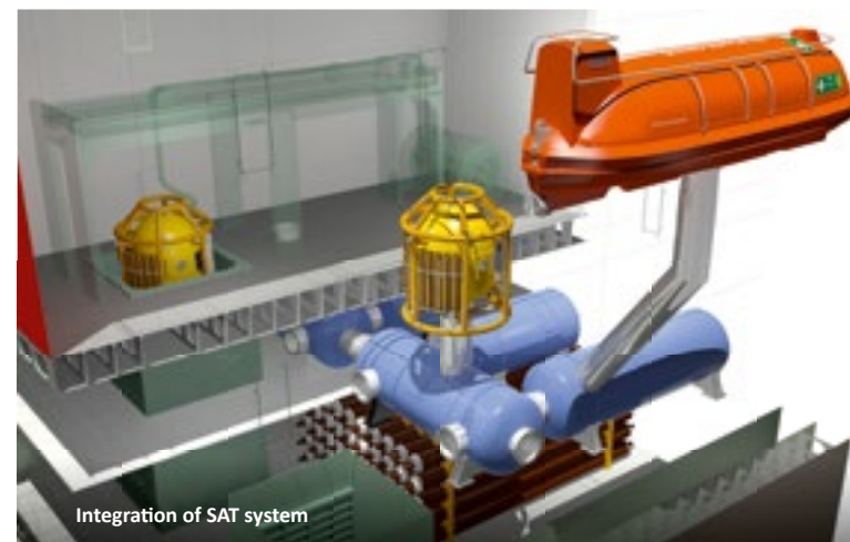
An 18-man integrated saturation diving system
