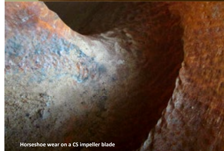
Wear at the trailing edge of a CS impeller blade after 15 million m 3
